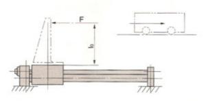
F: Drive (Position, lo from slide block) drag (kg) lo: Distance from mounting surface to load's center of gravity (cm)
